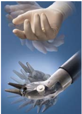
Hand of da Vinci robot (below) showing its greater dexterity compared with human hand.
